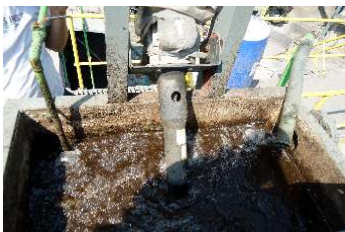
Pilot plant commissioned at M/s Star Paper mill, Saharanpur for the microbial effluent treatment process developed by CPPRI & IGIB
